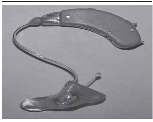
Figure 3. Illustration of the TransEar from Ear Technology Corporation. The digital signal processing hearing aid (upper) connects to the custom earmold (lower) via a wired link (available in seven lengths). In the earmold is a bone conduction receiver that transmits sound from the ear canal of the "dead" ear across the skull to the cochlea of the normal inner ear on the opposite side. Photo courtesy of Ear Technology Corporation. Used with permission.
