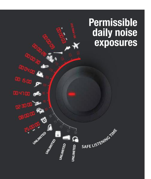
The permissible time for safe listening decreases as sound levels increase. This graphic explains the permissible daily noise exposures at different decibel (dB) levels. It shows examples of various levels of sound produced by different objects, highlighting the maximum safe listening duration in hours, minutes and seconds for each dB level. The daily recommended safe volume level of any sound is below 85 dB for a maximum duration of eight hours.
